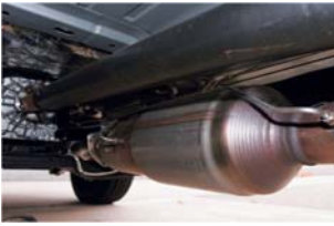
Installation of exhaust gas-reduction device
