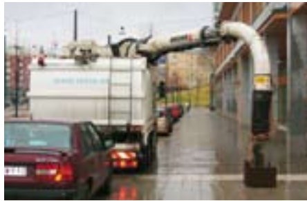
Refuse collection vehicle with vacuum suction system at one of the docking points for the mobile automated waste disposal system.
