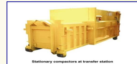
Stationary compactors at transfer station
