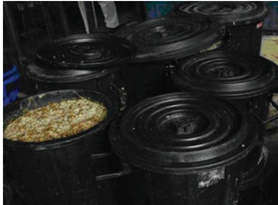
Picture 14. Trapped grease is used as additional fuel at slaughterhouse
